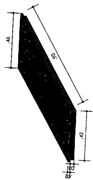
DETALHE DAS PLACAS DE CONCRETO
